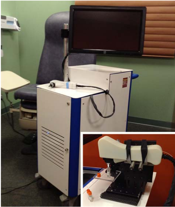
Figure 1 Handheld optical imaging system utilizing OCT. System is designed to be portable and can be easily transported to and from clinical sites. Handheld probe utilizes interchangeable tips to allow for both a wide field-of-view during benchtop imaging as well as compatibility with speculum tips used during human subject imaging. Inset: Handheld probe in a mounted configuration used to take measurements of phantom samples and aspirated ex vivo middle ear effusions.
