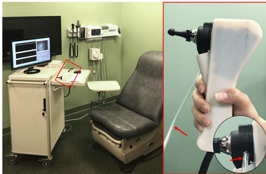
Fig. 2. The handheld probe uses a standard ear speculum with a rubber earbud to ensure a pressure seal within the ear canal. The pneumatic pressure stimulus is provided via a pneumatic port (bottom right) and surgical tube (red arrows).
