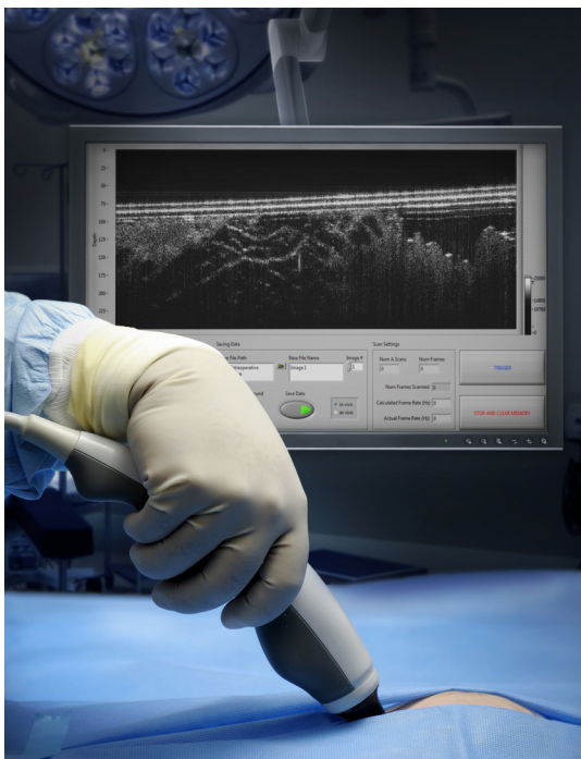
Fig. 1 Simulated representative intraoperative imaging scenario using an optical imaging-based hand-held probe for assessing the tumor cavity and resection bed. Advances are needed toward slide-free, stain-free, real-time, in vivo imaging during surgery to reduce positive margin and reoperation rates and to improve patient outcomes. Figure courtesy of Stephen Boppart, the Biophotonics Imaging Laboratory, and the Imaging Technology Group at the Beckman Institute for Advanced Science and Technology, University of Illinois at Urbana-Champaign, Urbana, Illinois.
