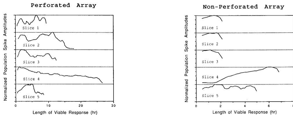
Fig. 4. Population spike amplitudes over time for rat hippocampal slices on perforated and nonperforated electrode arrays. (Note the significant difference between time scales.)
