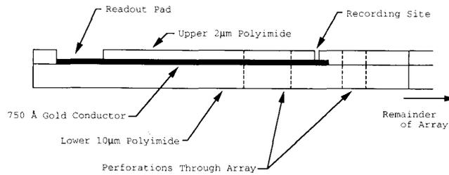
Fig. 1. Side view of a flexible perforated electrode array, in the absence of a rigid substrate, showing polyimide sandwich of Au/Ti conductor and RIE-formed holes and perforations.
