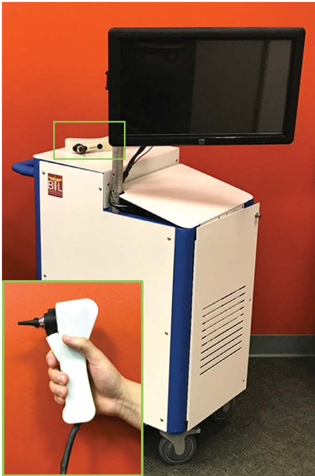
Fig. 1. Portable, hand-held, optical coherence tomography (OCT) system. Hand-held probe (green box and inset) of the custom-built portable OCT system resembles a standard otoscope. The head of a standard otoscope is integrated to utilize a disposable ear speculum.
