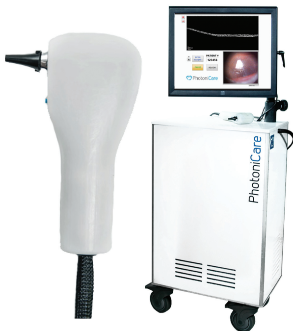
Figure 1. Photos of the prototype optical coherence tomography otoscope (left) and accompanying cart system (right). Three devices were designed, built, and clinically tested to successfully complete this pediatric middle ear infection study.
