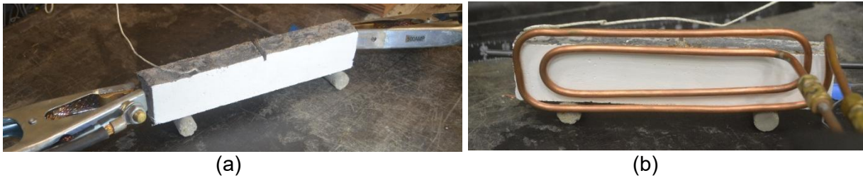
Fig. 13. Setup for heating using (a) electricity and (b) induction
