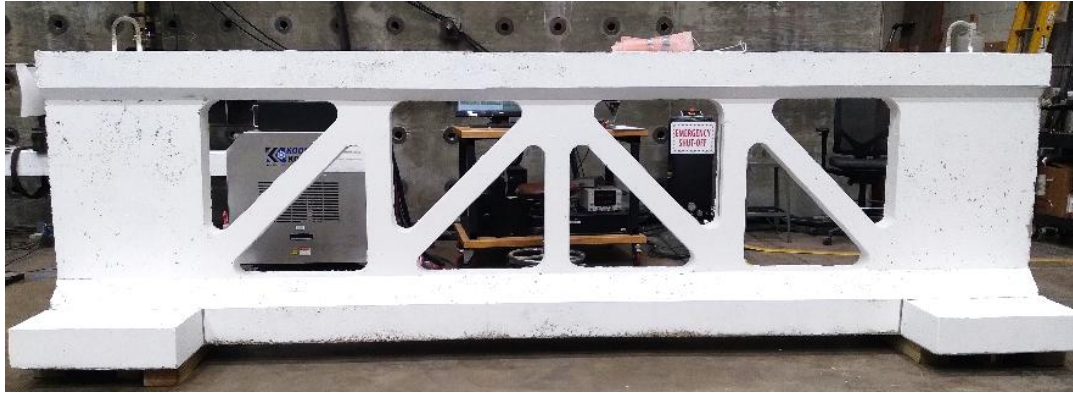
Fig. 26. Cured and painted concrete truss
