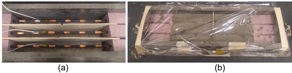
Fig. 11. (a) Formwork with SMA inside, and (b) formwork after concrete was poured
