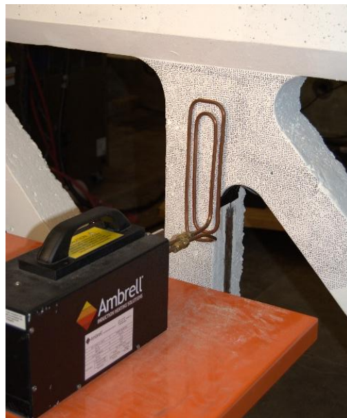
Fig. 27. Electromagnetic induction heating of the concrete vertical member
