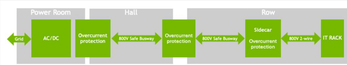
NVIDIA 800 VDC architecture minimizes energy conversions [1]
