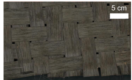
Figure 6. Optical microscopy on recovered fibers showing no significant resin deposition.
