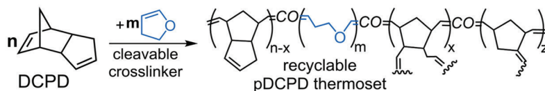
Figure 1. Copolymerization reaction between DCPD and DHF.
