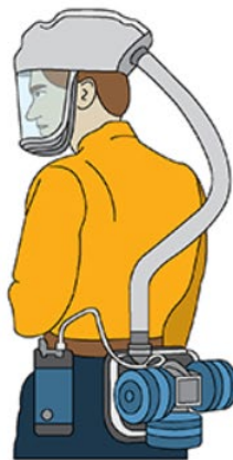
Loose-Fitting Powered Air-Purifying Respirator (PAPR) APF=25
