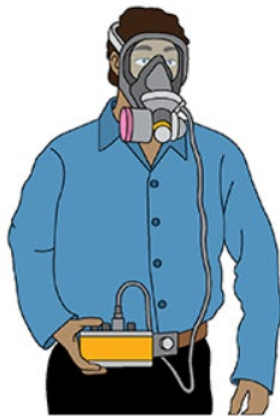
Tight-Fitting Full Facepiece Powered Air-Purifying Respirator (PAPR) APF=1,000 Needs to be fit tested
