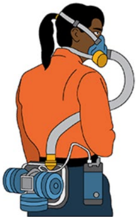
Tight-Fitting Half Facepiece Powered Air-Purifying Respirator (PAPR) APF=50 Needs to be fit tested
