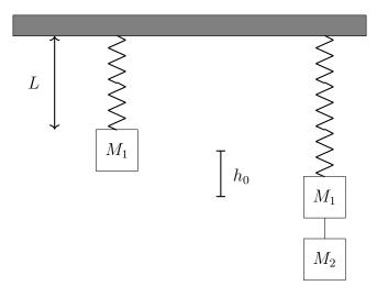
Since all the forces acting on the blocks are conservative (spring and gravity), we can use energy conservation. The total potential energy stored in the spring initially is given by
