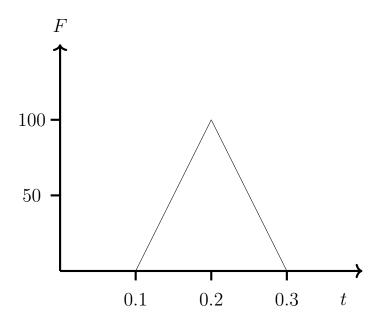
Impulse is given by  $\Delta P = F_{ave}\Delta t$ . We find  $F_{ave}$  by taking the integral of the Force function and dividing by the change in time.
