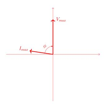
We know that in order to get the current, we would need to project  $I_{max}$  onto the y-axis. Since we know the angle  $\phi$ , we are able to calculate this projection:
