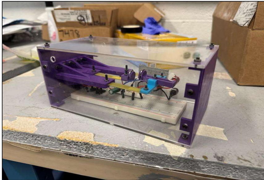
Figure 9: Final Piezoelectric Energy Harvesting Assembly within Housing
