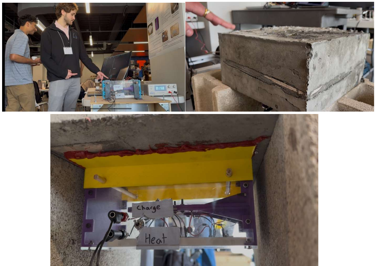
Figure 18. Mechanical Science and Engineering student design team capstone presentation (top left), the cast concrete bridge deck specimen with the embedded nichrome wire (top right) and the energy harvesting piezoelectric system under the bridge deck specimen (bottom)
