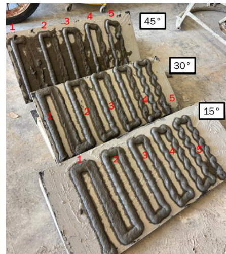
Figure 1. Experimental validation of nozzle height effects on filament deposition quality across planar inclined surfaces
