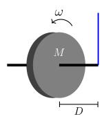
The angular momentum of the spinning disk is  $L=124 \text{ kgm}^2/\text{s}$ . The time it takes the gyroscope to make one complete revolution in the horizontal plane (its precession period) is 22.2 seconds.
