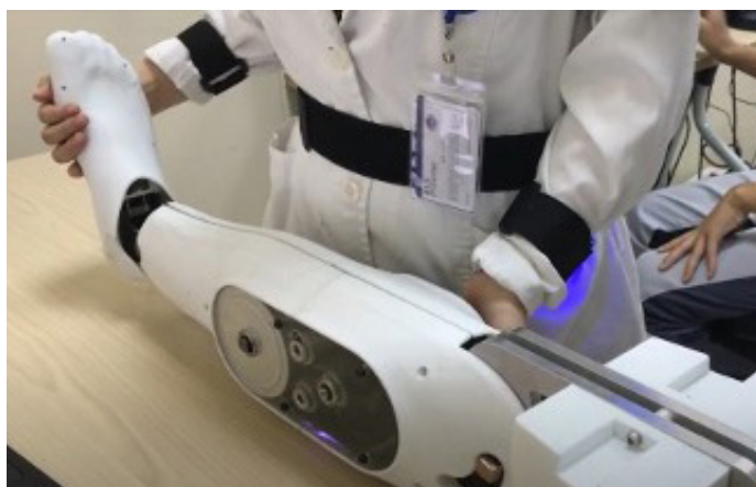
Hsiao-Weckler’s medical education task trainers - in this case, robotic limbs that can provide haptic feedback to medical students who are training to perform neurological exams.
