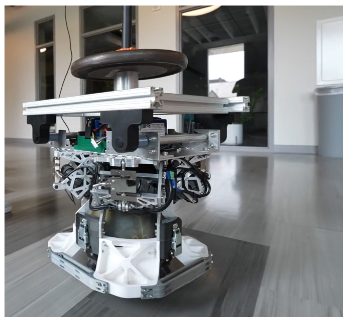
The PURE ball-based mobility device (Gen3 seen here) can carry payloads over diverse terrain, setting the stage for more adaptive transport for patients experiencing limited mobility.
