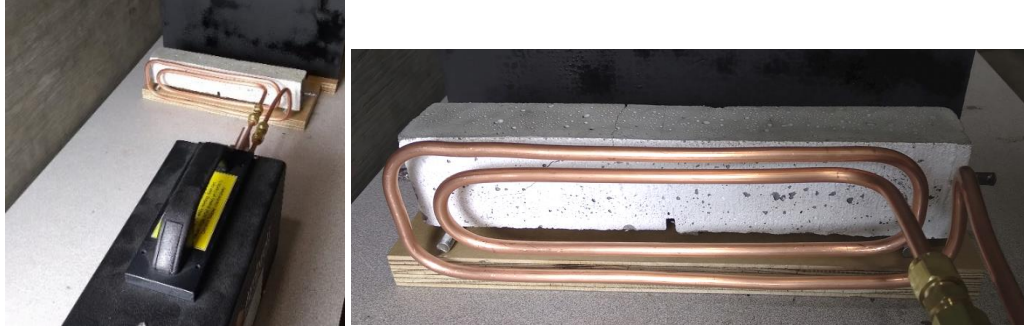
Figure 9. Induction coil with practice test specimen
