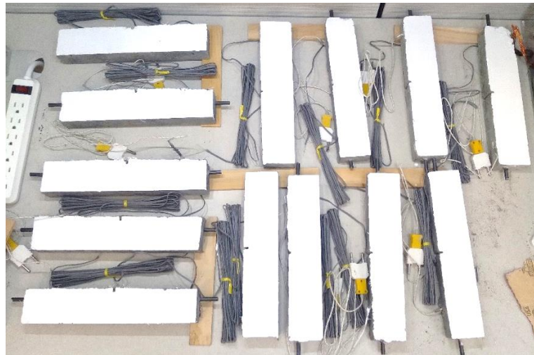
Figure 8. Flexural specimens with instrumentation
