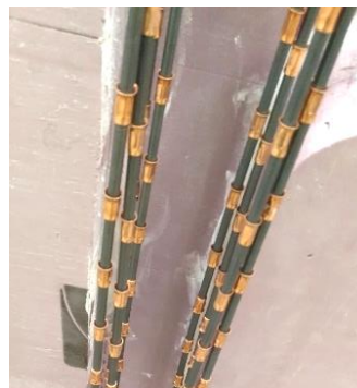
Figure 5. Close-up of SMA alloy with crimps
