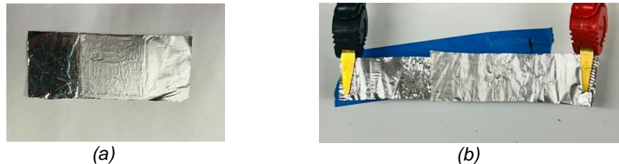
Fig. 1 Capacitor. (a) A square capacitor with metal leads protruding in opposite directions. (b) Capacitor with metal leads connected to the LCR meter by two electrical clips.
