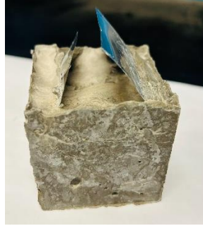
Fig. 2 A capacitor embedded in cement, with electrical leads in the form of steel foils protruding from the cement.
