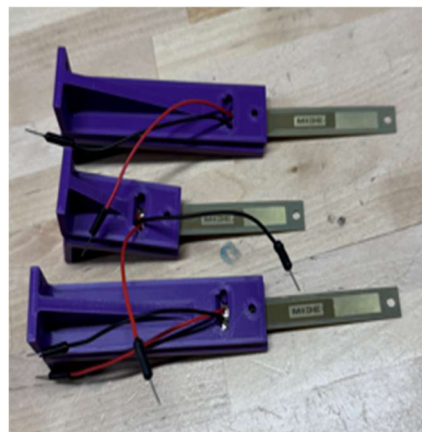
Figure 6. Piezoelectric harvesters in the mounts
