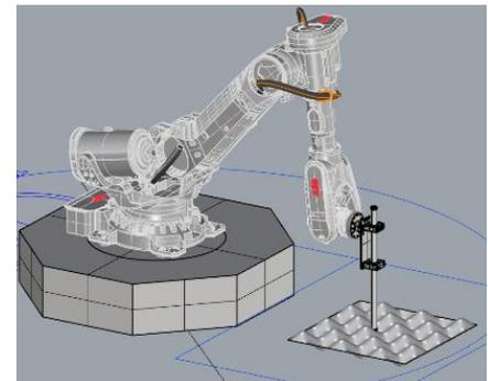
Figure 4. Integration of the generated surface and toolpath within the ABB IRB6700 robotic arm environment.
