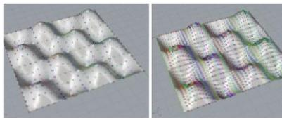
Figure 2. Point distribution over the parametrized surface used for toolpath generation. Increasing the number of points refines the mesh, enabling greater geometric complexity and improved alignment with printing parameters such as nozzle diameter.
