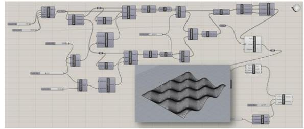
Figure 1. Grasshopper definition implemented to parametrize and slice the sinusoidal surface geometry.
