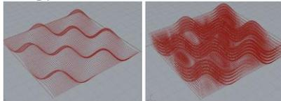
Figure 3. (a) Interpolated curves generated through surface points and connected at endpoints to form a continuous toolpath. (b) Layered array of connected curves defining the complete multi-layer toolpath for additive manufacturing.
