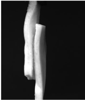
Lap-shear test (ASTM D5868)
