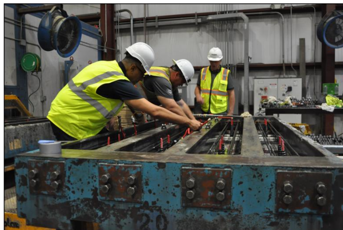
Figure 6. TRANs-IPIC researchers and Rocla Concreet Tie staff during the process of fabricating the crossties with SMA reinforcement.
