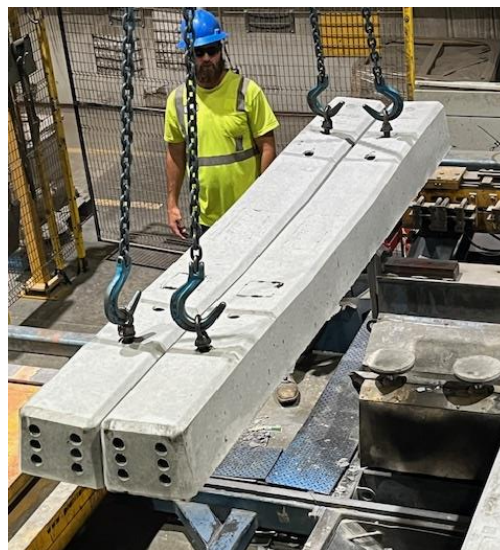
Figure 6. TRANs-IPIC researchers and Rocla Concreet Tie staff during the process of fabricating the crossties with SMA reinforcement.
