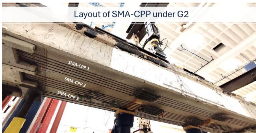
Fig 6. Image of ongoing Shape Memory Alloy-Coupled Prestressing Plates (SMA-CPP) large-scale test at UIUC.
