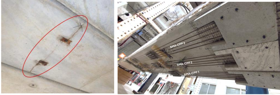
Figure 12. Innovative technique for externally prestressing bridge girders proposed by TRANS-IPIC researchers using smart materials.
