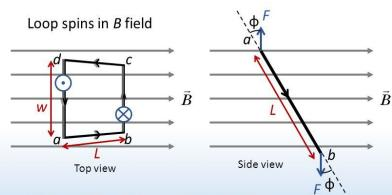
B field generates a torque on the loop
