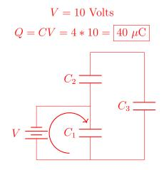
(ii) Capacitor 2 and 3 are in series, so combine capacitors 2 and 3 in series using the equation
