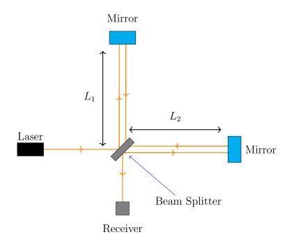
What is the minimum increase in  $L_2$  required so that only 100 W goes to the detector? (Note that when the arms are of equal length, the detector receives 200 W).
