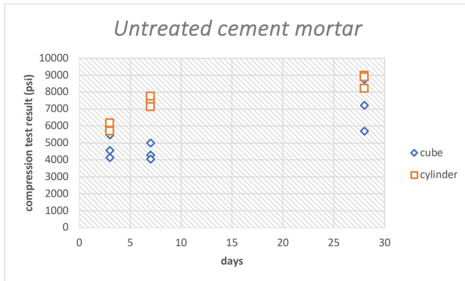
Figure 12. Compression test result of untreated cement mortar.
