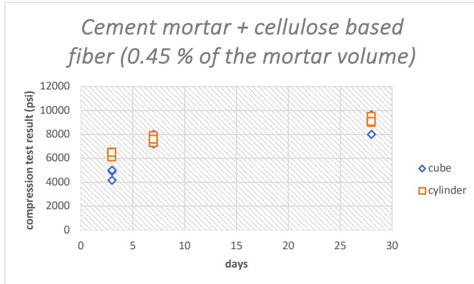
Figure 13. Compression test result of cement mortar with cellulose fiber.
