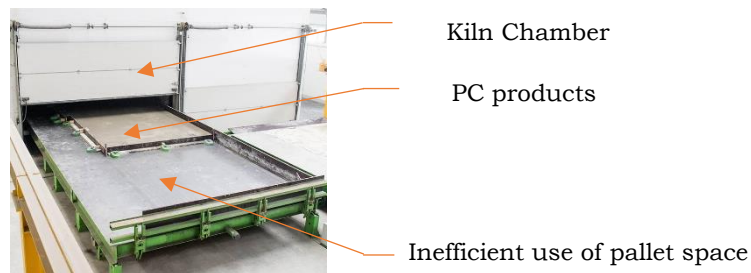
Figure 3. Mold placement on a pallet in curing process
