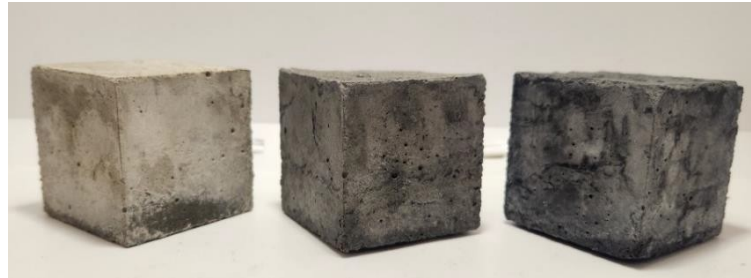
Figure 3. From left to right; reference, rCB1, and rCB2 mortar samples.
