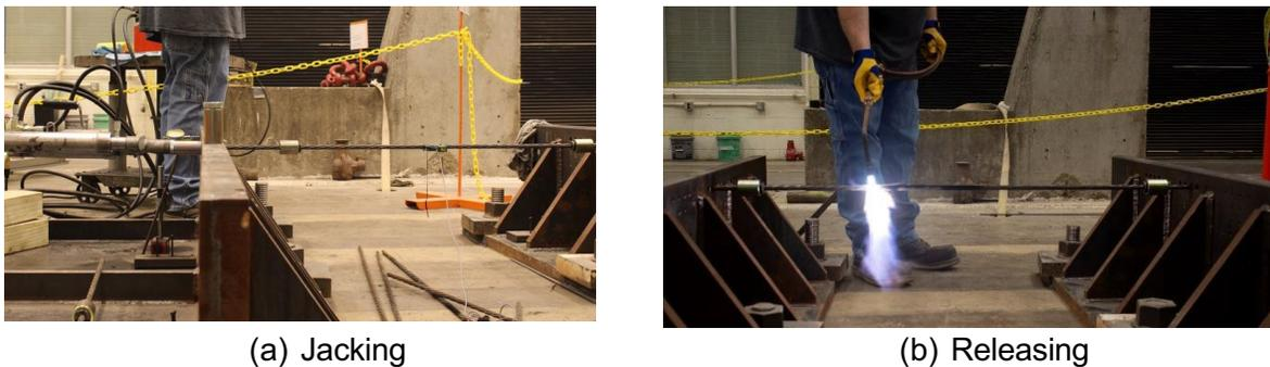
**Figure 6.** Pre-tensioning process of a prestressing strand
