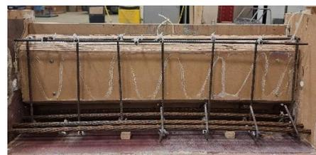
(b) Steel and wood mold assembly
