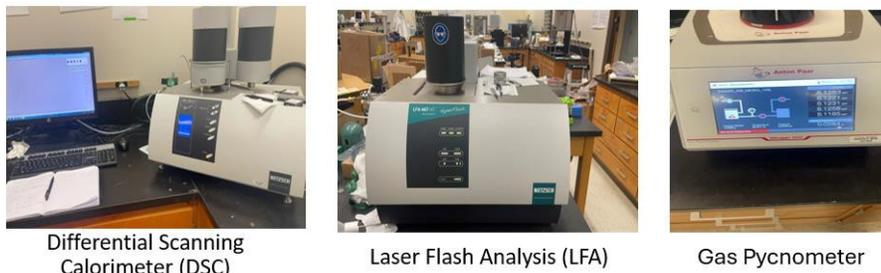
Differential Scanning Calorimeter (DSC)
