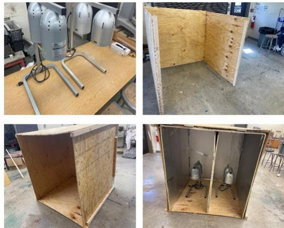
**Figure 3:** Reflective Thermal – Insulated Box Preparation
