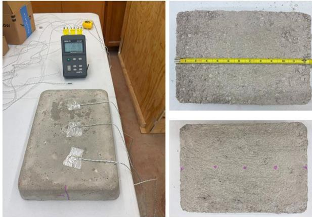
**Figure 4:** Marking and Installing Thermocouple Sensors on Top and Bottom Surfaces.
