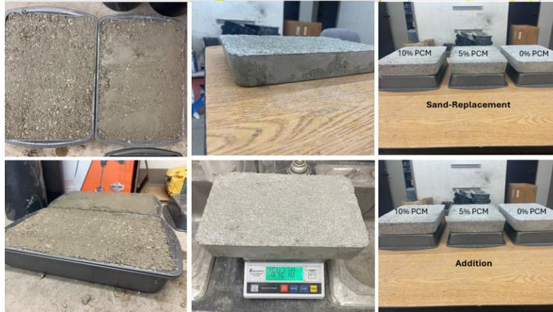
**Figure 2:** Concrete - PCM samples with 0%, 5% and 10% by addition and by Sand-Replacement.
