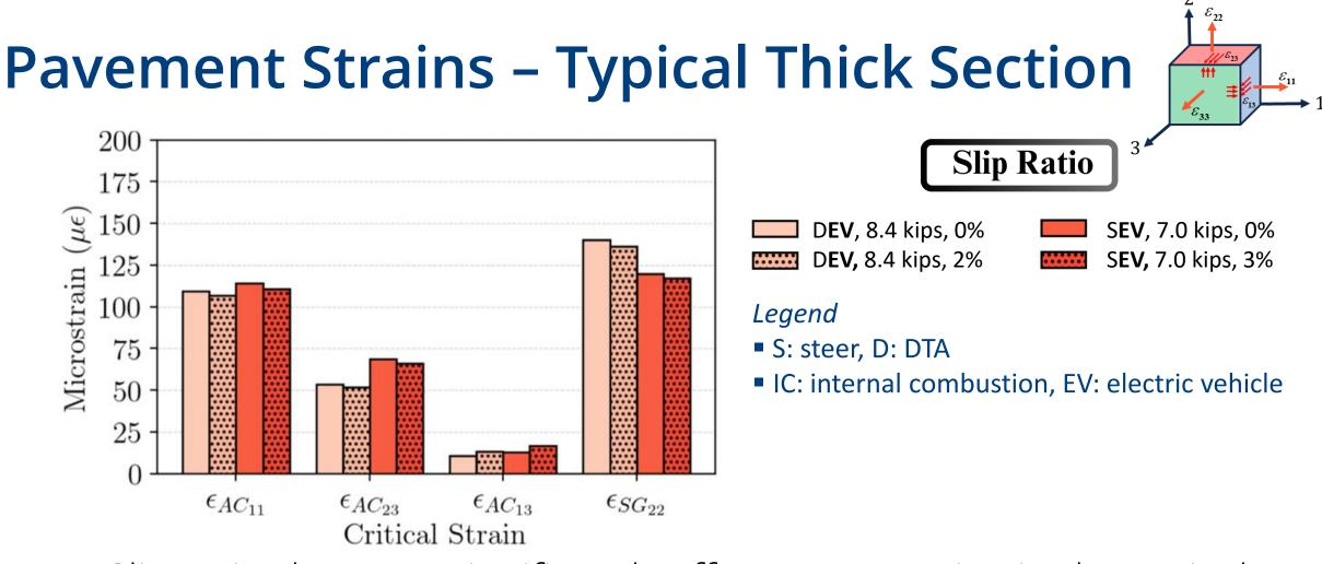
Slip ratio does not significantly affect most strains in the typical thick pavement section
