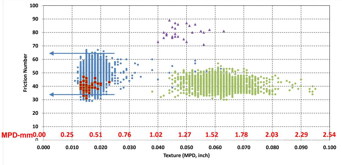
Source: FDOT, 2013. • Dense • Open • Concrete (Longitudinal Grinding) • HFST
