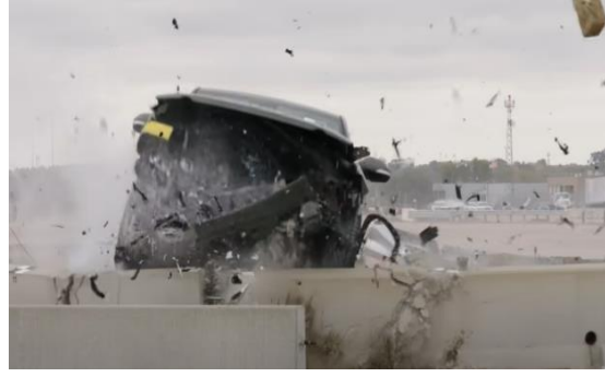
Fig-1. A 7,000-pound Rivian R1T truck crushed and tore through concrete barriers commonly used as freeway median barriers or to shield highway construction workers from ongoing traffic, with minimal deceleration, posing significant risks to both passengers and infrastructure [1][2].
