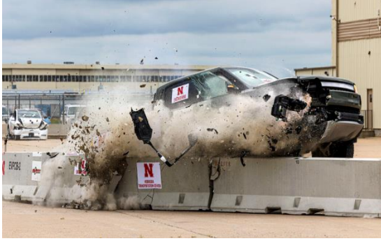
Fig-1. A 7,000-pound Rivian R1T truck crushed and tore through concrete barriers commonly used as freeway median barriers or to shield highway construction workers from ongoing traffic, with minimal deceleration, posing significant risks to both passengers and infrastructure [1][2].
