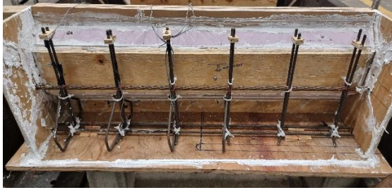
(a) Steel stirrup specimen
