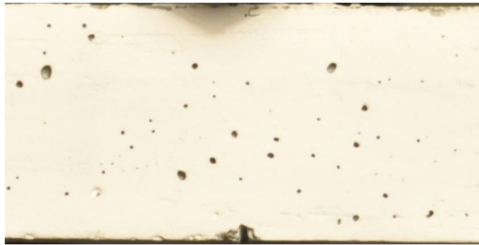
Figure 7. Crack after second SMA activation
