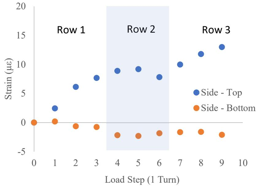
Figure 12: Measured strain as a function of tightening of 3 rows of 0.375 in. anchors
