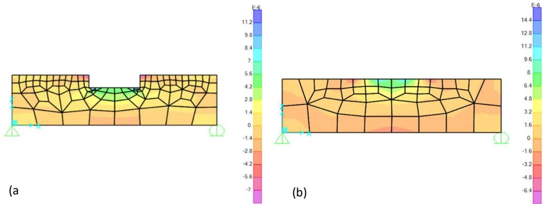
**Figure 5:** Strain field for maximum lateral force of (a) lab jack and (b) 0.25 in anchors.
