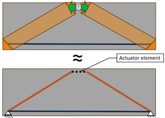
**Figure 3:** Comparison of a strut-and-tie concrete model with compression struts (orange) and tension ties (blue) due to applied load [top]. The dynamic relaxation formulation has axial elements in the same color scheme with an additional actuator element (black dashed) to simulate the expanding anchor or jack.
