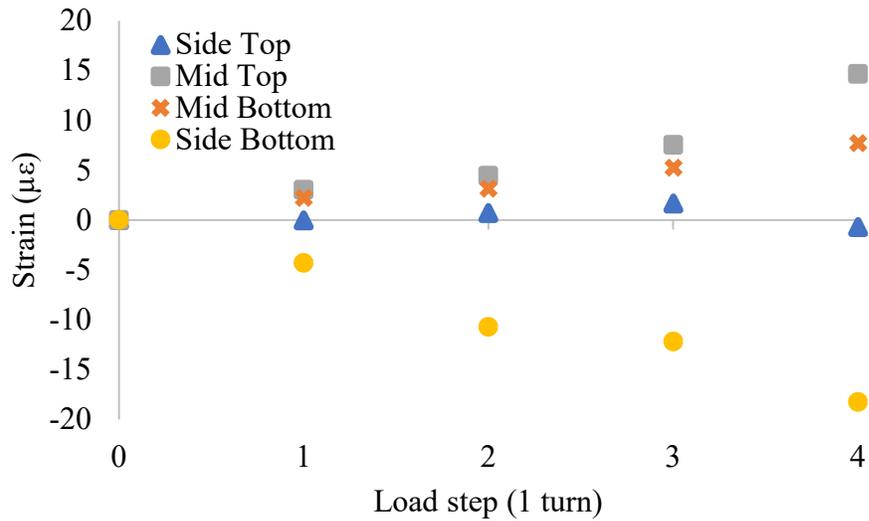
Figure 13: Measured strain as a function of tightening the 0.375 in. anchor.
