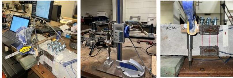
Figure 14: Deployable a 3 rows of 9-0.375 in. anchors being installed into the concrete specimen 4 [left]. LVDT displacement/voltage data collecting [center] and front view of the anchor installation with and LVDT sensor on specimen 4 [right].
