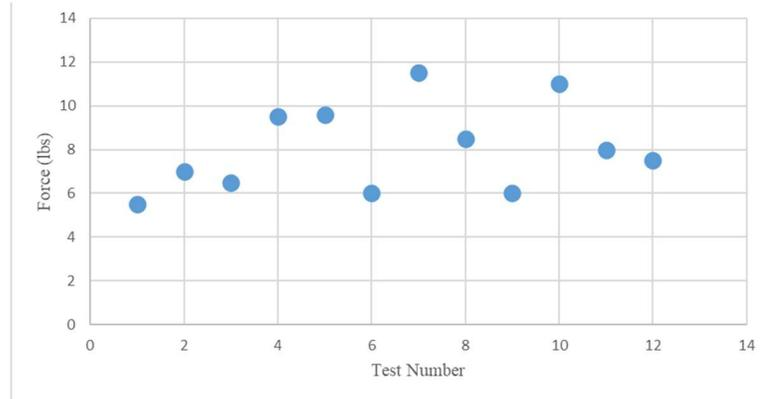
**Figure 6:** Lateral Force Capacity for the Hollow-Wall Anchors
