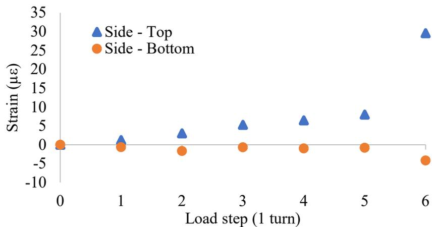
Figure 11: Measured strain as a function of tightening the 0.25 in. anchor.
