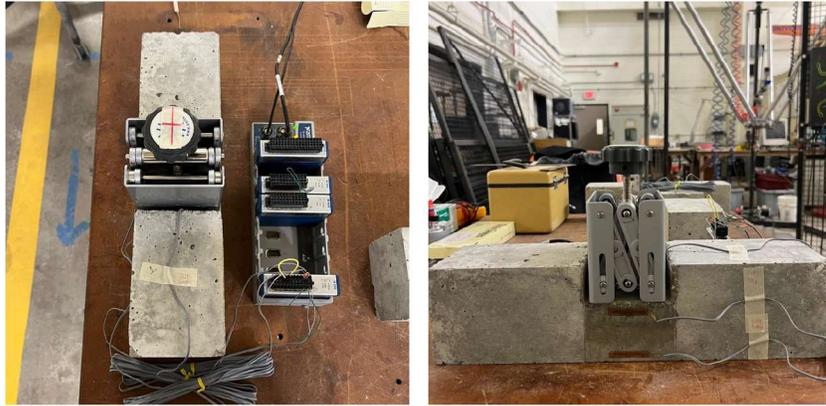
Figure 8: Experimental setup with the lab jack as the actuator.
