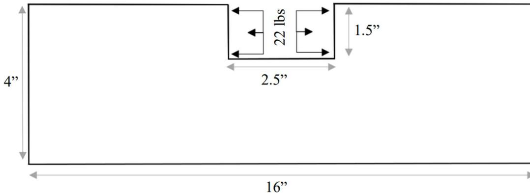
**Figure 4:** Elevation view of the concrete specimen with the maximum compressive force available from the lab jack to be applied in the compression zone for adaptive camber.
