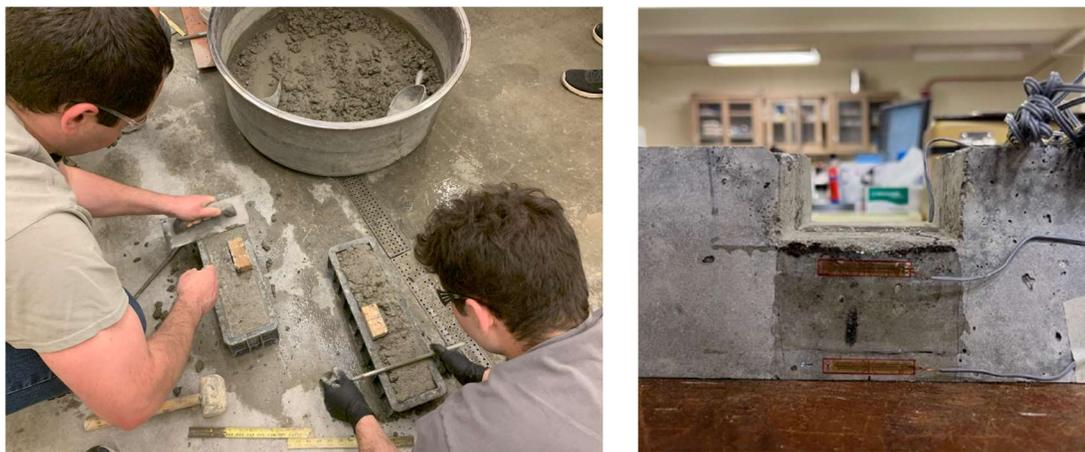
**Figure 7:** Casting of concrete specimens [left] and instrumentation [right].
