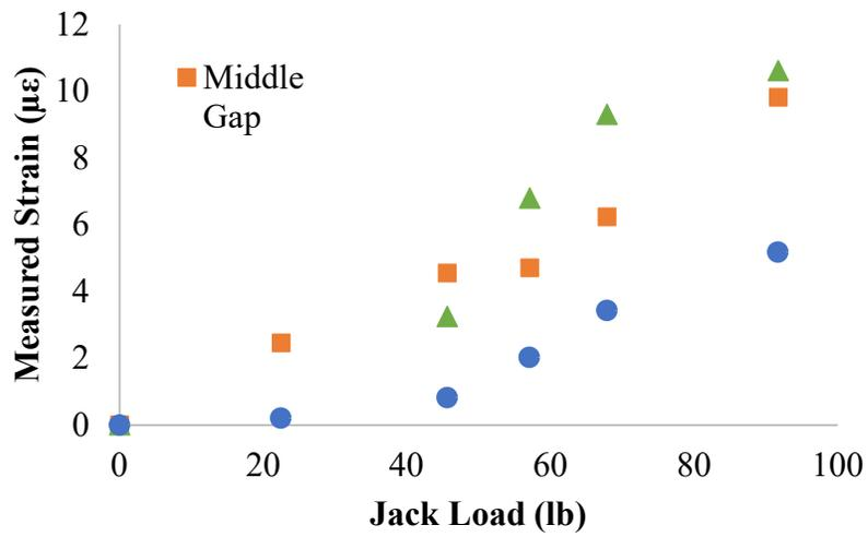
Figure 9: Measured strain as a function of the applied load from the lab jack.
