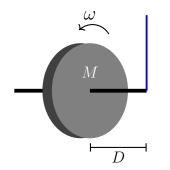
The angular momentum of the spinning disk is  $L = 124 \text{ kgm}^2/\text{s}$ . The time it takes the gyroscope to make one complete revolution in the horizontal plane (its precession period) is 22.2 seconds.
