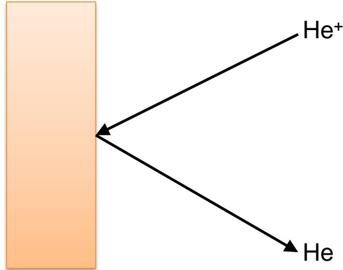
**RBS is an analytical technique where high energy ions (~2 MeV) are scattered from atomic nuclei in a sample. The energy of the back-scattered ions can be measured to give information on sample composition as a function of depth.**
