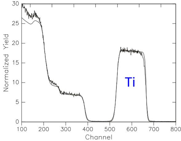
Experimental spectra and simulated spectra by RUMP
