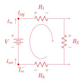
$-15 + R_1 I_{battery} + R_2 I_1 + R_3 I_{battery} = 0$
