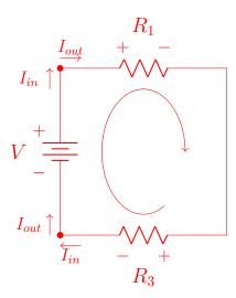
Using a KVL equation, we find that the new current through  $R_3$  is
