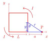
We have to define an angle  $\theta$  to relate dl and r in the cross product. From the diagram above,  $r = \sqrt{a^2 + y^2}$  and  $d\vec{l} \times \hat{r} = dy \sin(\theta)(-\hat{z})$ Where  $\sin(\theta) = \frac{a}{\sqrt{a^2 + y^2}}$
