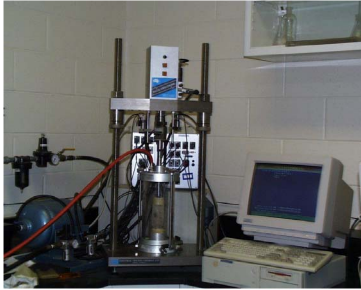
FIGURE 2.5 Photograph Showing Small Triaxial Test Setup at ATREL.
