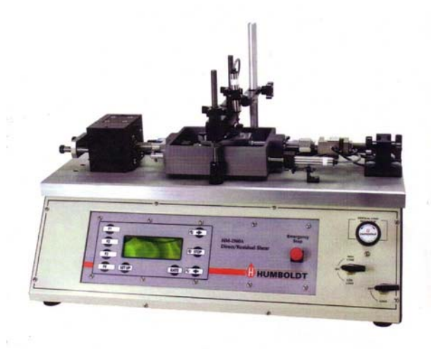
FIGURE 2.6 Assembly of Humboldt Pneumatic Direct Shear Testing Device.
