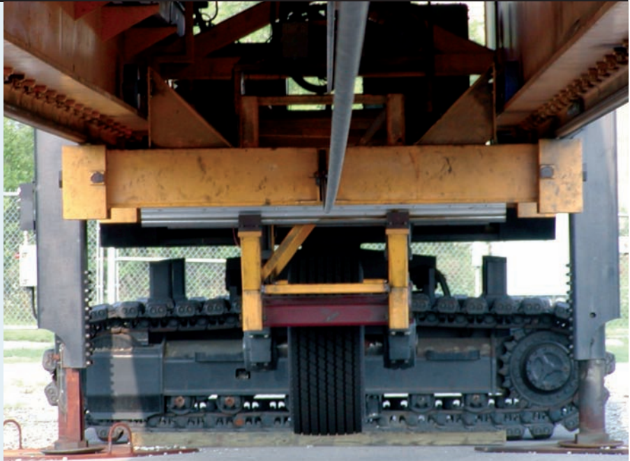
The US$2 million Accelerated Transportation Loading System can apply 10,000 repetitions per day
