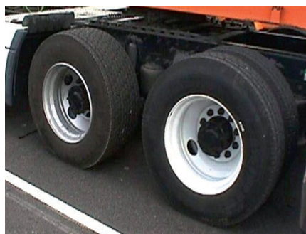
Wide-base tires being tested on Smart Road
