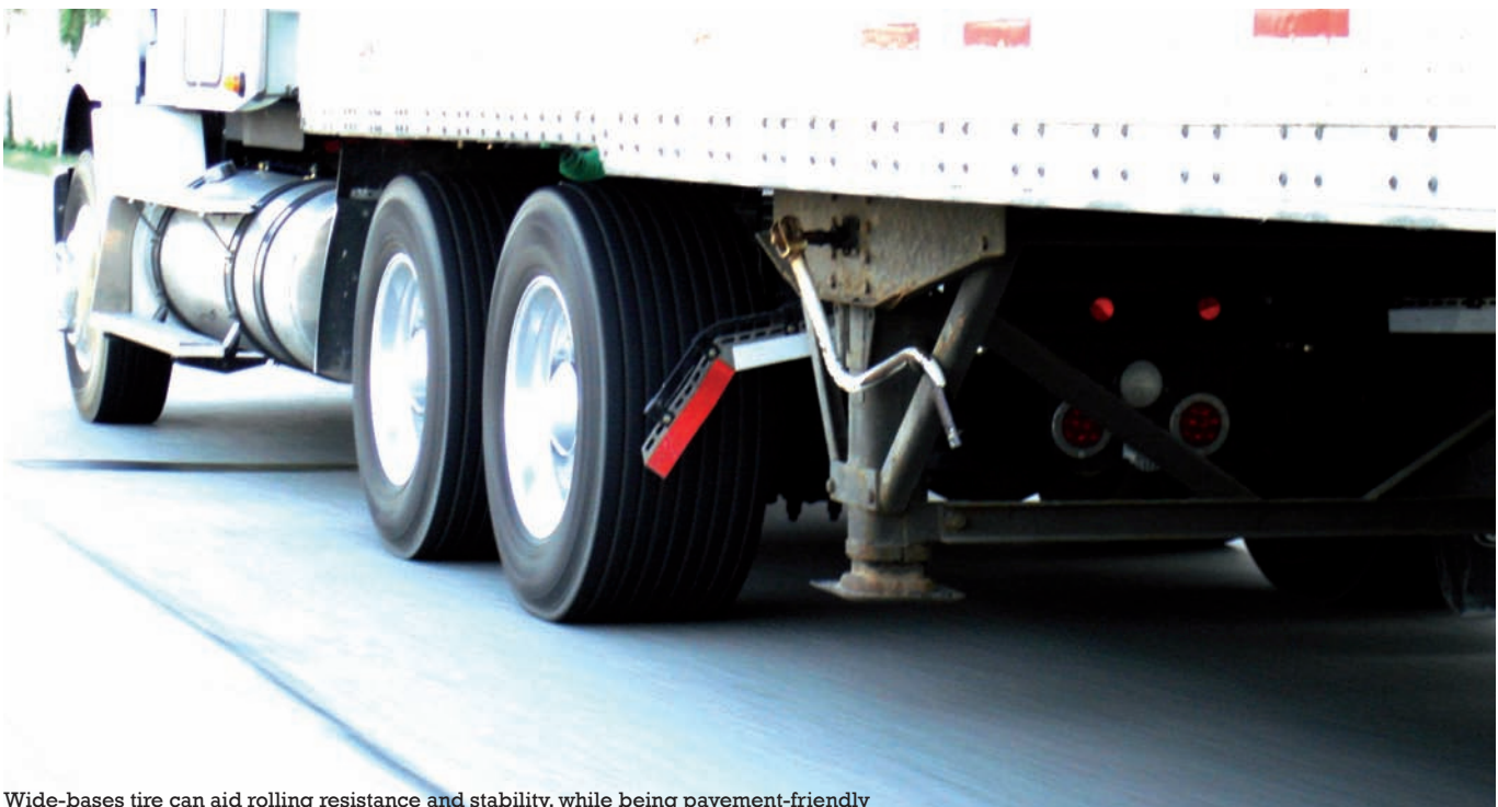
Wide-bases tire can aid rolling resistance and stability, while being pavement-friendly
