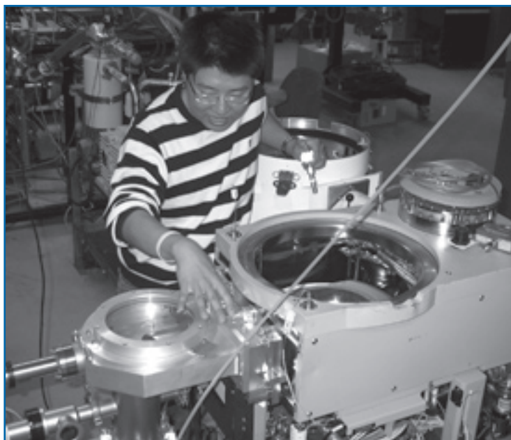
Graduate student Hyungjoo Shin works with a device used to put metal wire into computer chips. Novellus, Inc., donated the equipment to Prof. David Ruzic's laboratory.
