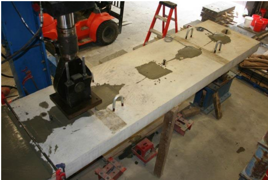
Figure 1. Photo. After grouting large-scale beam specimen 4F1.
