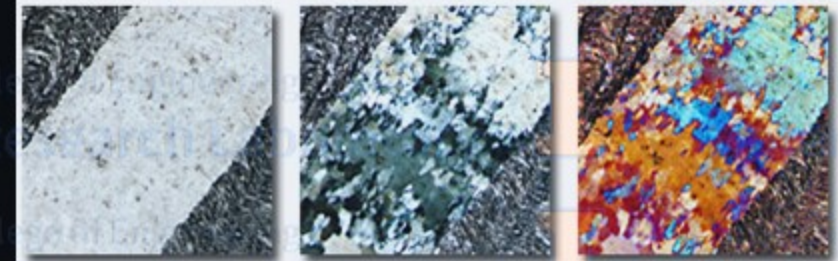
Phyllite Thin Section in Polarized Light
