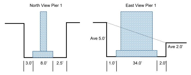
Per Article 502.12 (b): "Horizontal dimensions will not extend beyond vertical planes 2 ft outside of the edges of footings..."
