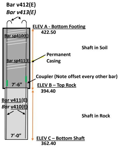
Calculate the volumes of concrete in the drilled shaft per Art 516
