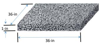
One Square Yard of HMA One Inch Thick Weighs 112 Pounds for Limestone and Dolomite Mixes
