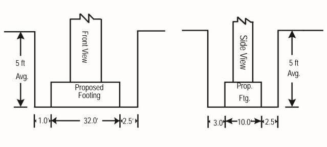
Determine the correct volume of Structure Excavation that will be used as final payment to the contractor at this location.
