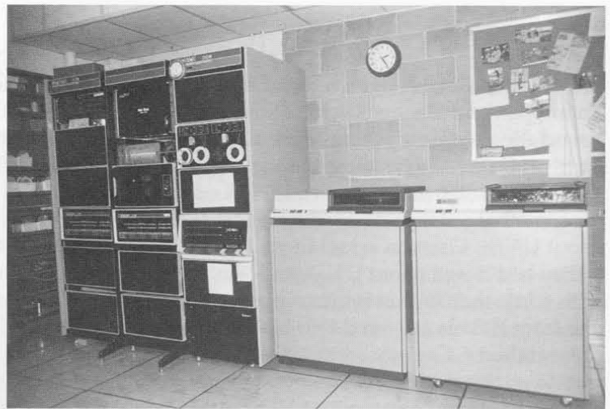
The first departmental "CRL machine," a PDP-11/45 (actually a /35—an OEM model), along with the two IBM 2314 29MB removable disk drives (the "washing machines").
