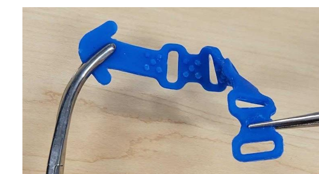
Fig. 7 Forceps can twist device without slipping
