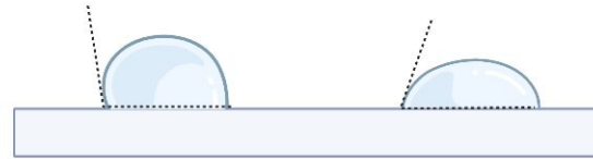
Fig 3. Water droplet test to measure hydrophobicity
