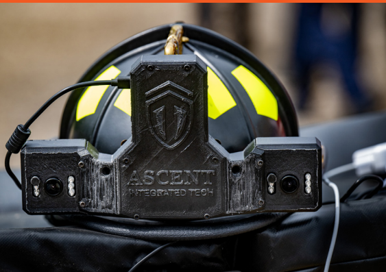
A firefighter's helmet carries the prototype set of front facing sensors as the team tests out their equipment.
