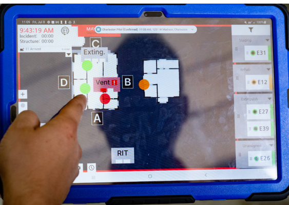
The Shield software displays real-time data so that incident commanders can access an event real-time, tracking when an operator is in distress.
